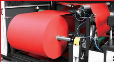
放料自动纠偏 Unwinding Auto Rectifying Deviation
