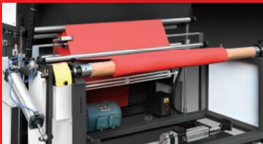
收料自动纠偏 Rewinding Auto Rectifying Deviation
